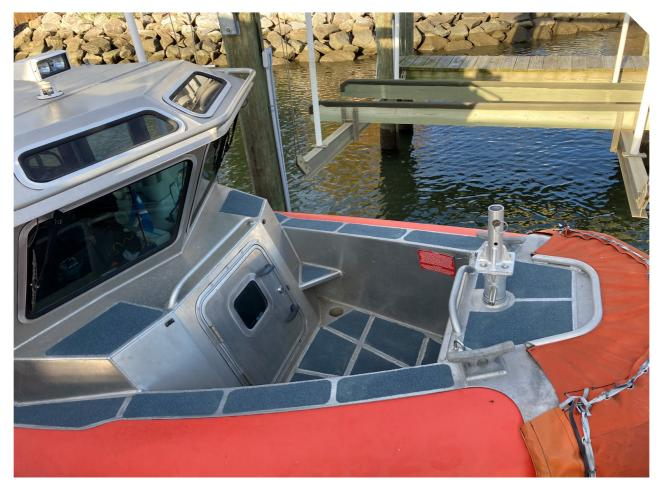
In addition, another epoxy formulation designed to increase traction on stairs and ladders, called Form-A-Tread Original, was applied in specific areas such as the vessel operator's footrest.
