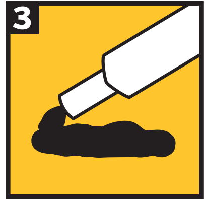
3 Screw on Mix Nozzle. Dispense and discard first 2 inches of material.
