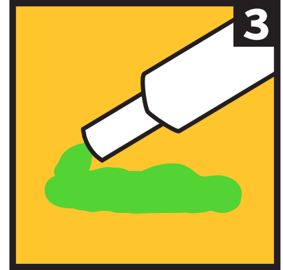
Attach mixing nozzle. Dispense first 2 inches of material.
